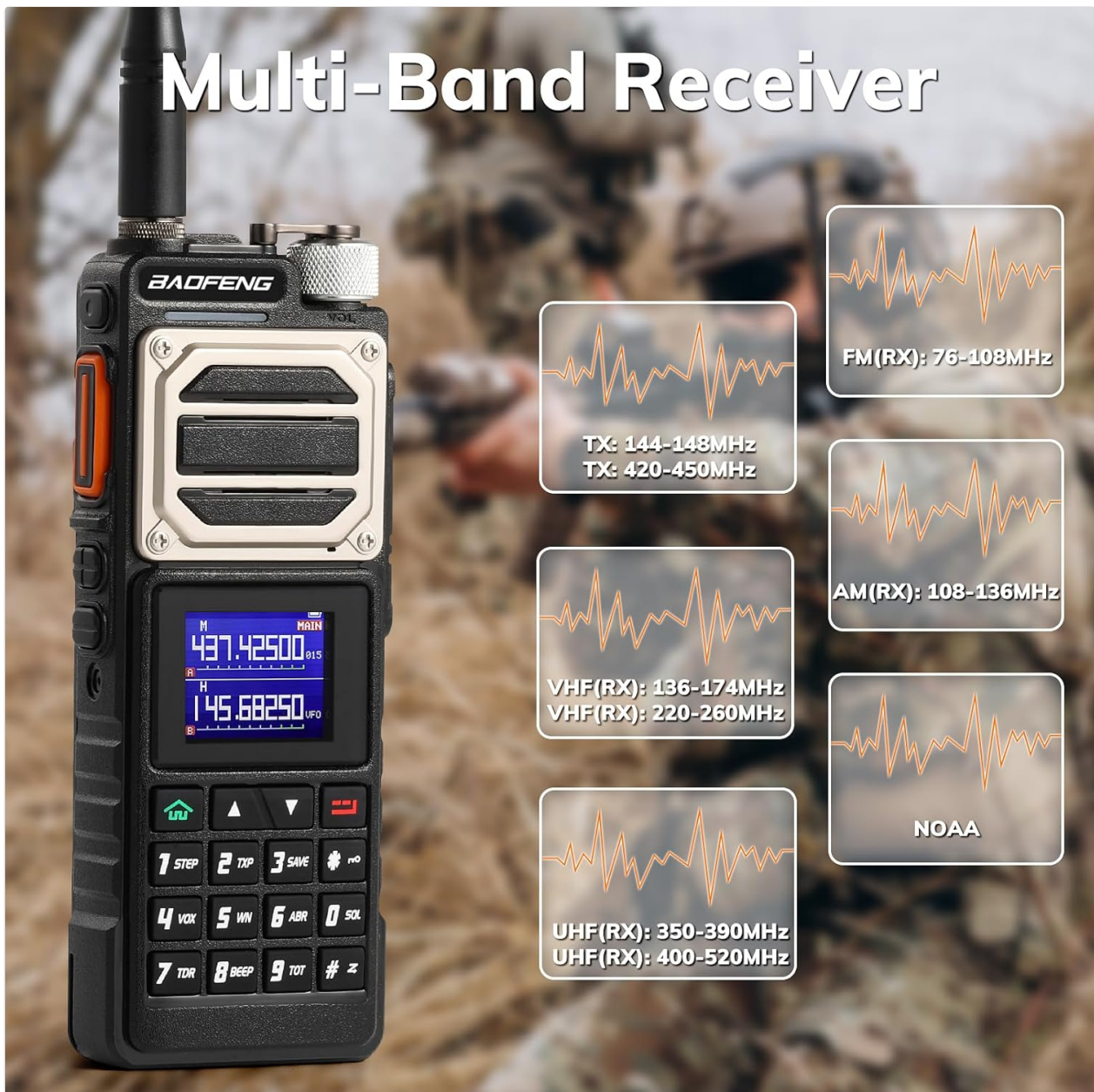
Figure 2: The BAOFENG UV-25 supports a wide range of reception frequencies, including FM, AM, VHF, UHF, and NOAA weather channels.
