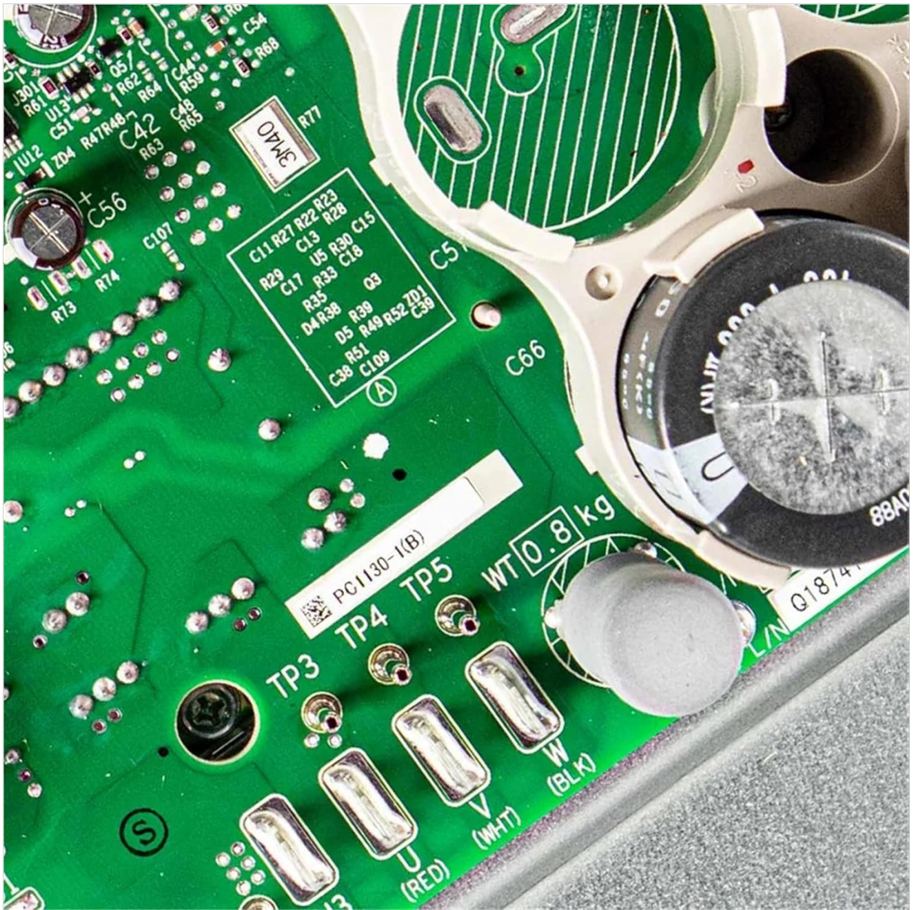
Image 3: Close-up of specific components and markings on the PC1130-1 PCB. This detailed view shows test points (TP3, TP4, TP5), weight marking (WT 0.8 kg), and other circuit details, including the "PC1130-1(B)" model identifier.
