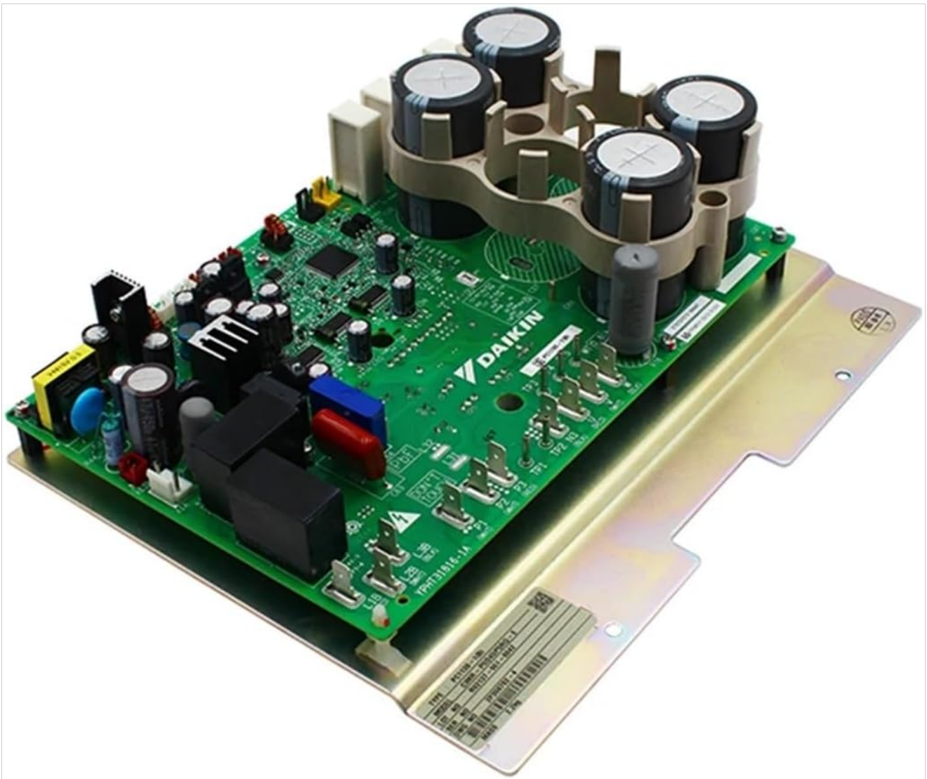
Image 2: Angled view of the PC1130-1 inverter PCB. This perspective highlights the large capacitors and other power components, providing a clearer view of the board's depth and component density.
