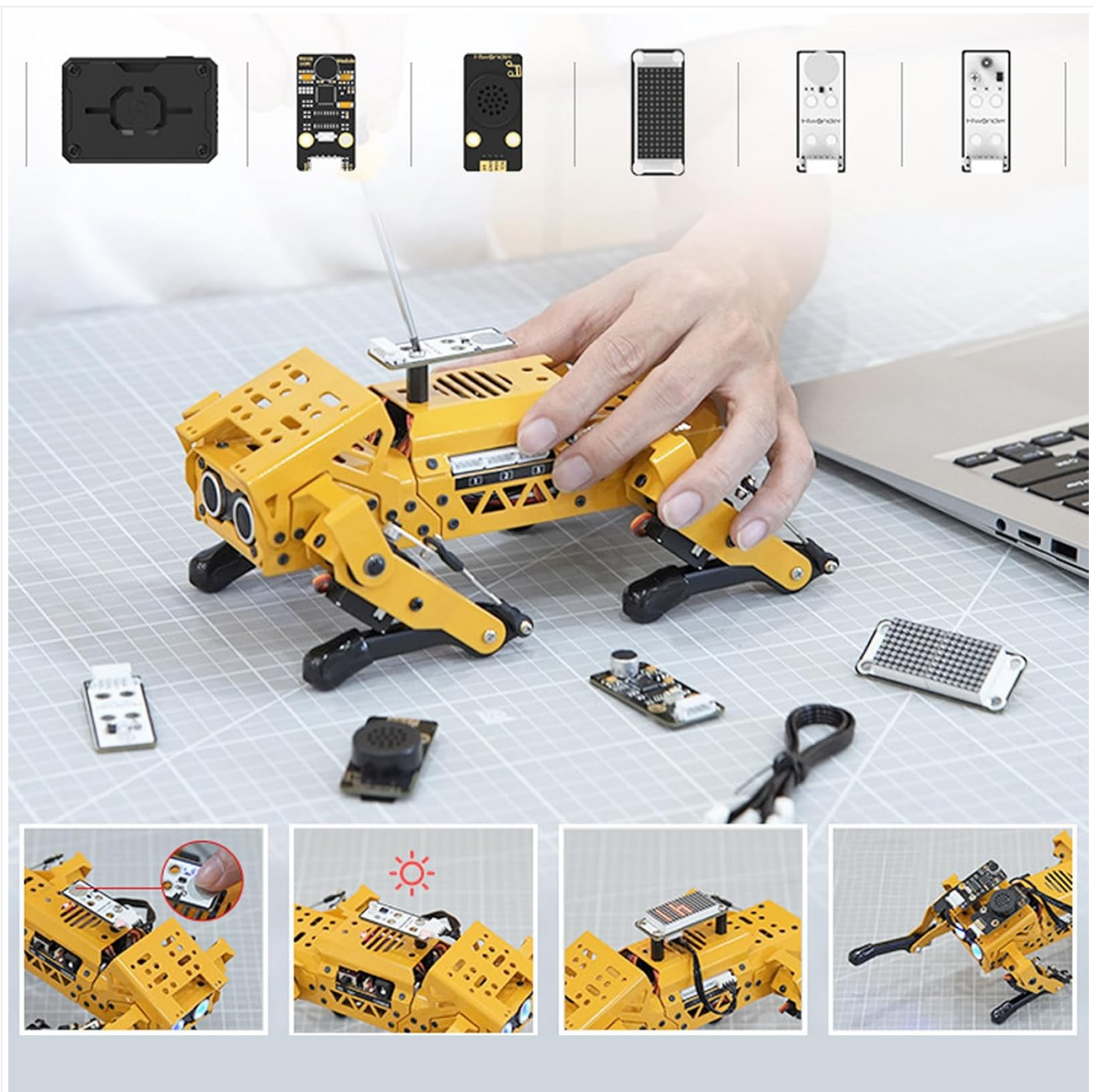
Image: Demonstrating the installation of an expansion module onto the robot dog.
