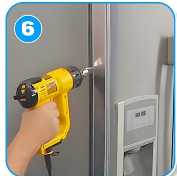
Strengthen the seal with a hair dryer
