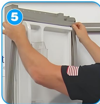
Install, press inwards from the corners
