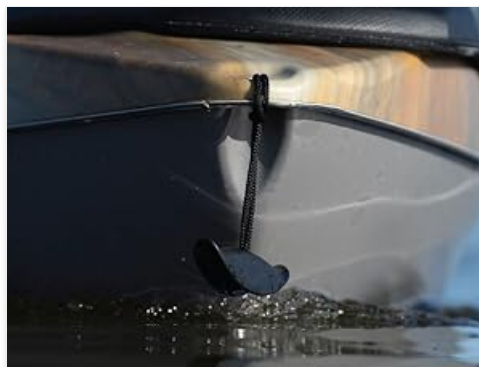
Figure 3.1: One of the four carrying handles, located at the stern for easy transport.
