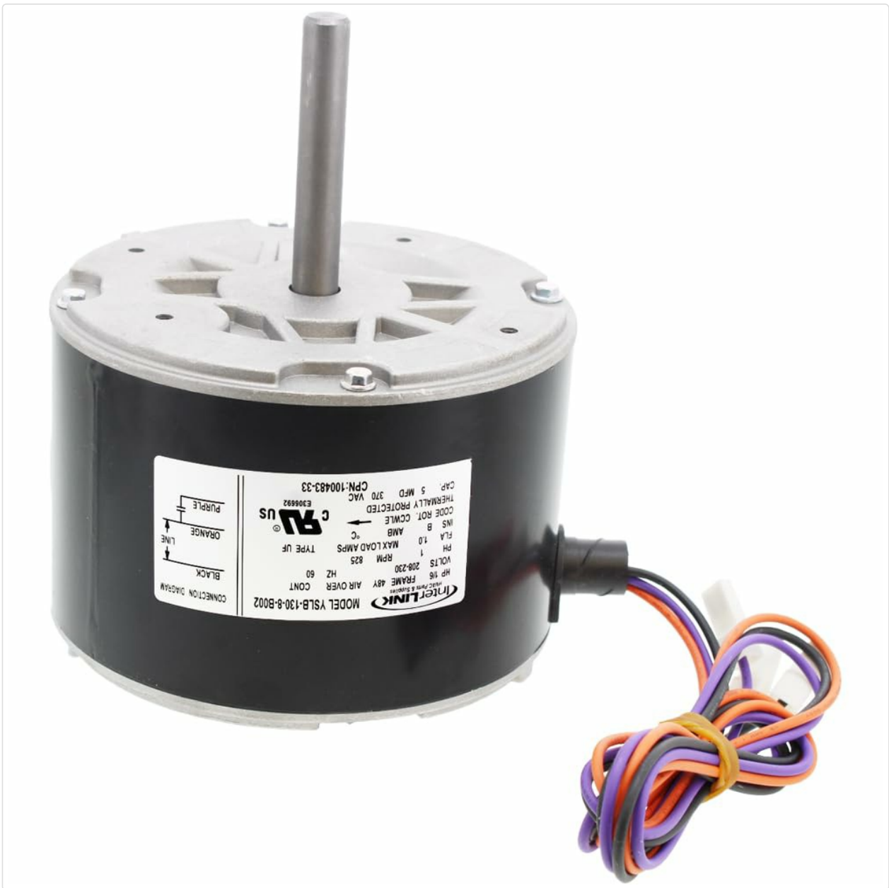
Figure 1: ClimaTek OEM Upgraded Condenser Fan Motor. This image displays the black motor with a grey top and a central shaft. A white label on the side provides detailed specifications, including the model number YSLB-130-8-B002, 1/6 HP, 825 RPM, 208-230V, and a connection diagram. A bundle of purple, orange, and black wires extends from the motor, ready for connection.
