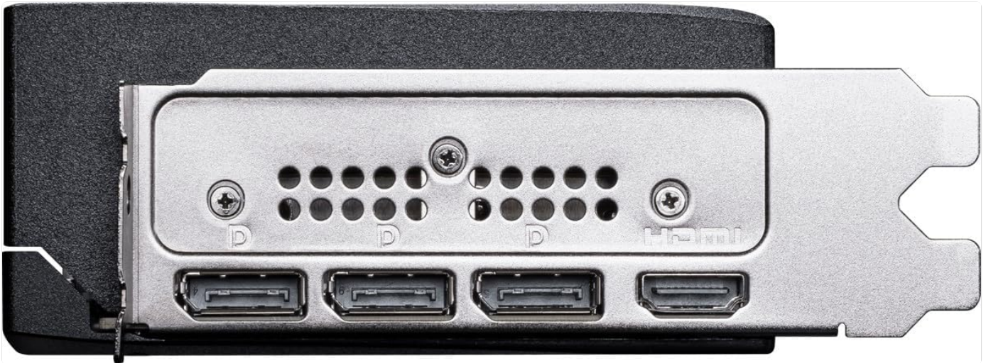
Figure 4.3: Rear I/O panel with DisplayPort and HDMI connectors.
