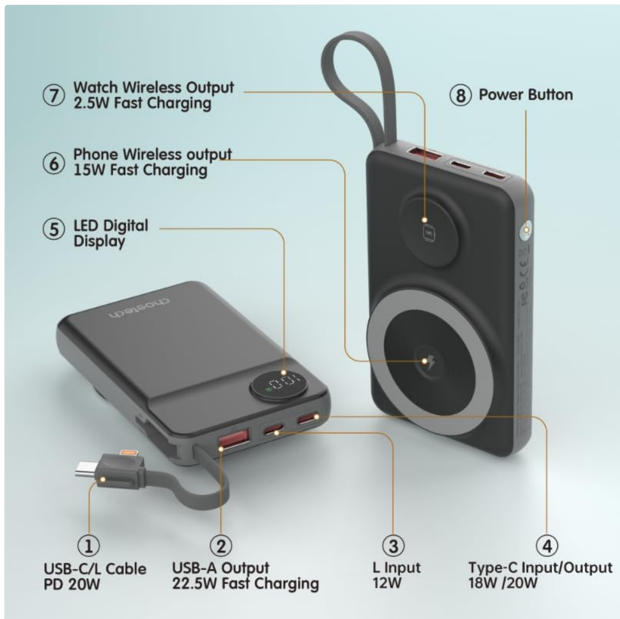
Image: Detailed diagram labeling the ports and features of the CHOETECH B695, including USB-C/L cable, USB-A output, L input, Type-C input/output, LED display, phone wireless output, watch wireless output, and power button.
