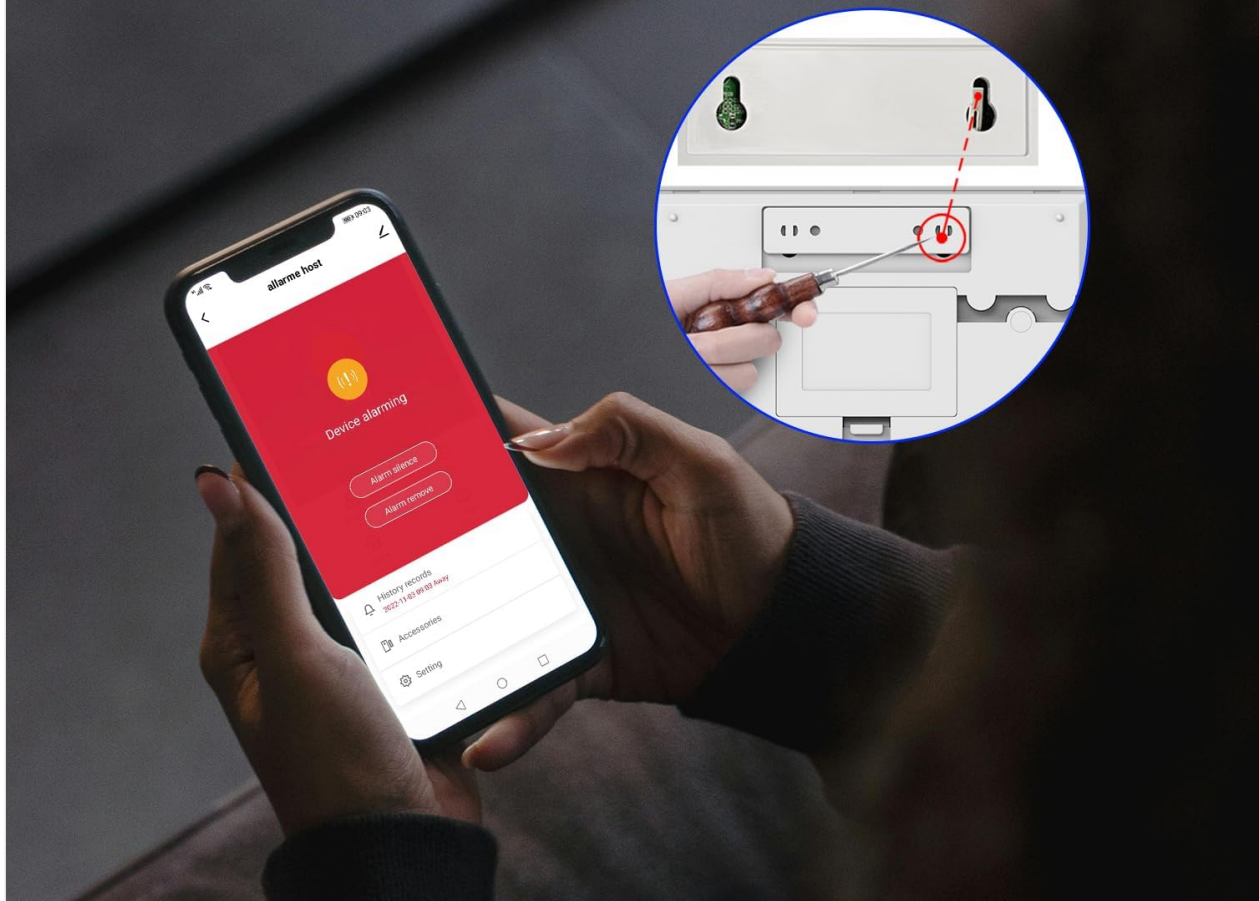
Figure 4.5: The anti-demolition feature provides an additional layer of security by alerting you if the main panel is tampered with.
