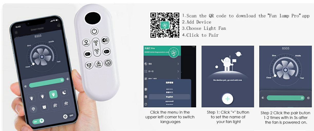
Image 5.3: Instructions for setting up app control, including a QR code to download the "Fan Lamp Pro" app, steps for adding a device, and pairing the fan with the app.
