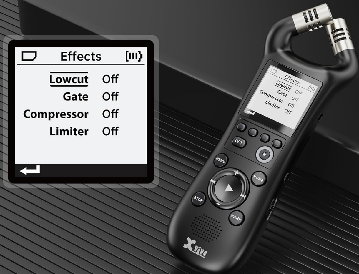
Image 5.5: The Effects menu on the Xvive XV1-R, showing options for Lowcut, Gate, Compressor, and Limiter.
