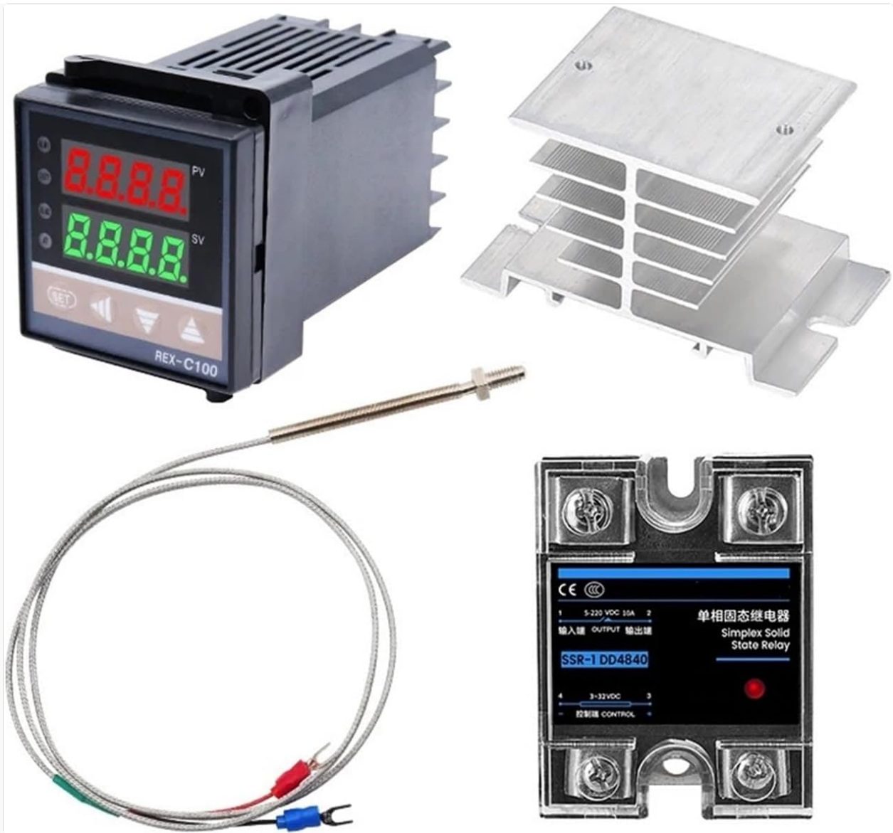
Image 2.1: Overview of the REX C100 PID Temperature Controller kit, showing the REX C100 unit, a K-type thermocouple, a solid-state relay (SSR), and an aluminum heatsink.
