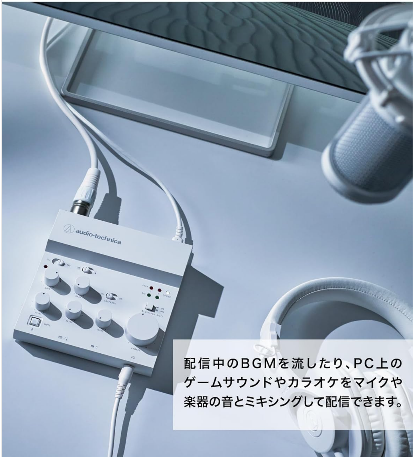
Figure 6: The Loopback switch allows mixing computer audio with live inputs.
