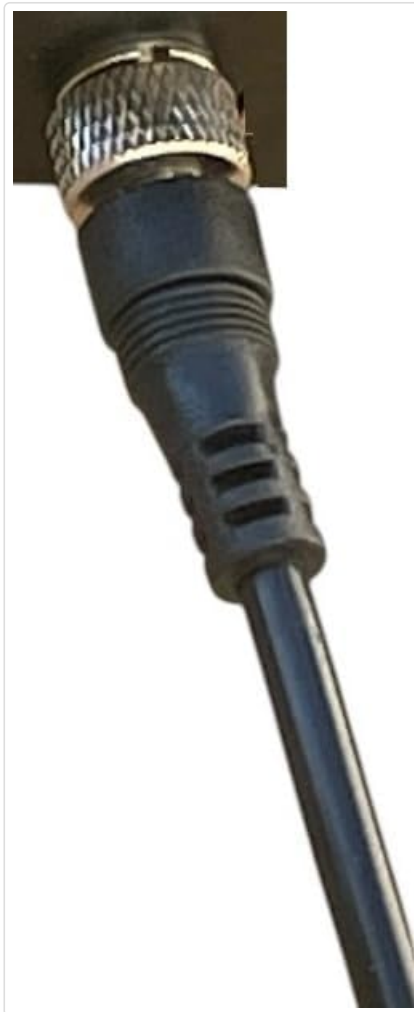
Figure 3.4: The locking DC output connector shown securely inserted into a compatible power input port.
