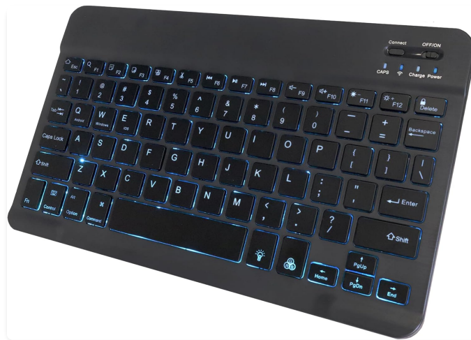
Image 2.2: A detailed view of the SlimKeys keyboard, showing the 'Connect' button and indicator lights for power, charge, and Bluetooth status.
