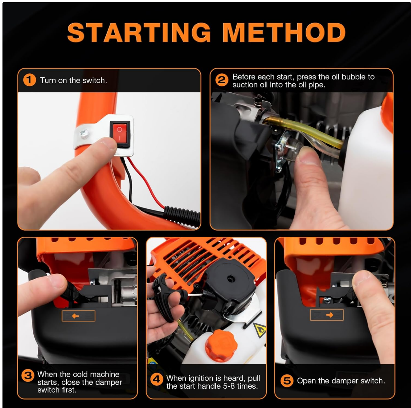
Figure 4.1: Engine starting method.
