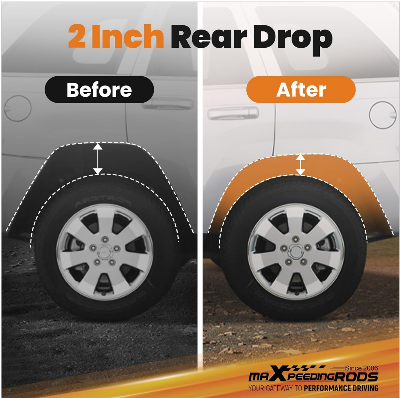
Image: Visual comparison demonstrating the 2-inch rear drop achieved by installing the lowering springs.
