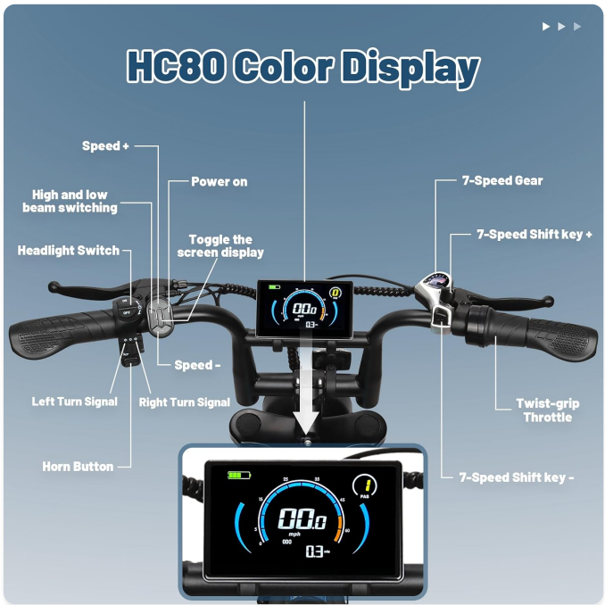
Image: Close-up of the HC80 color display and handlebar controls, including light switches, turn signals, and horn button.
