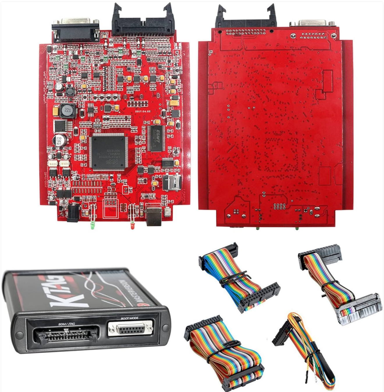
Figure 4: Internal view of the KTAG V7.020 Red PCB, along with various ribbon cables used for connecting to ECUs.
