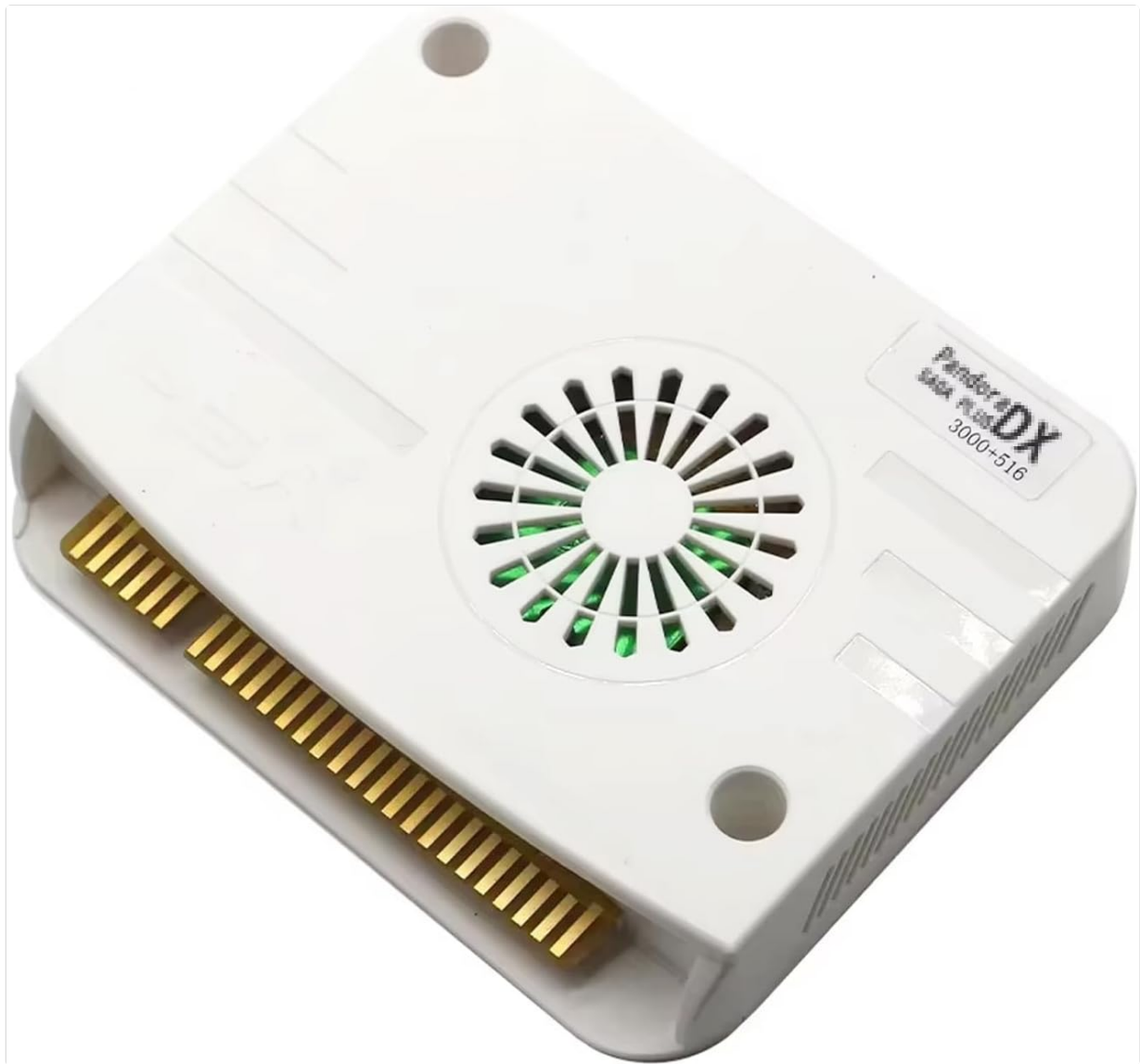
Image 1: The main PCB unit of the UYXOERA 3D Saga DX Plus Arcade System. This compact white box houses the core electronics and features a fan for ventilation, along with a multi-pin connector for integration into an arcade cabinet or control panel.
