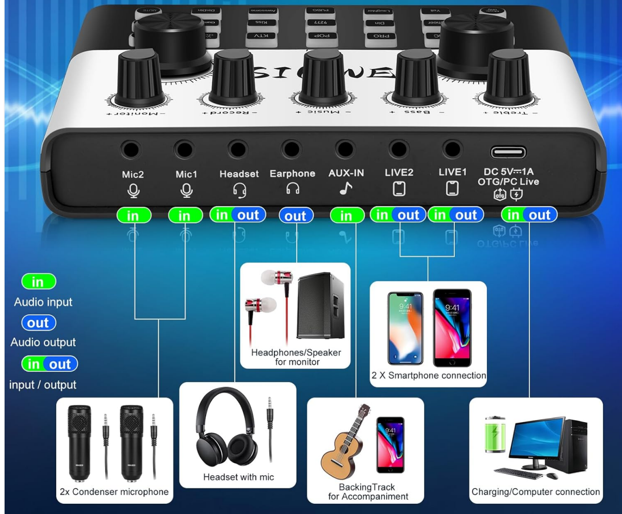
Image: Detailed connection diagram illustrating how to connect two microphones, headphones, a backing track, and two smartphones for dual-device live streaming.
