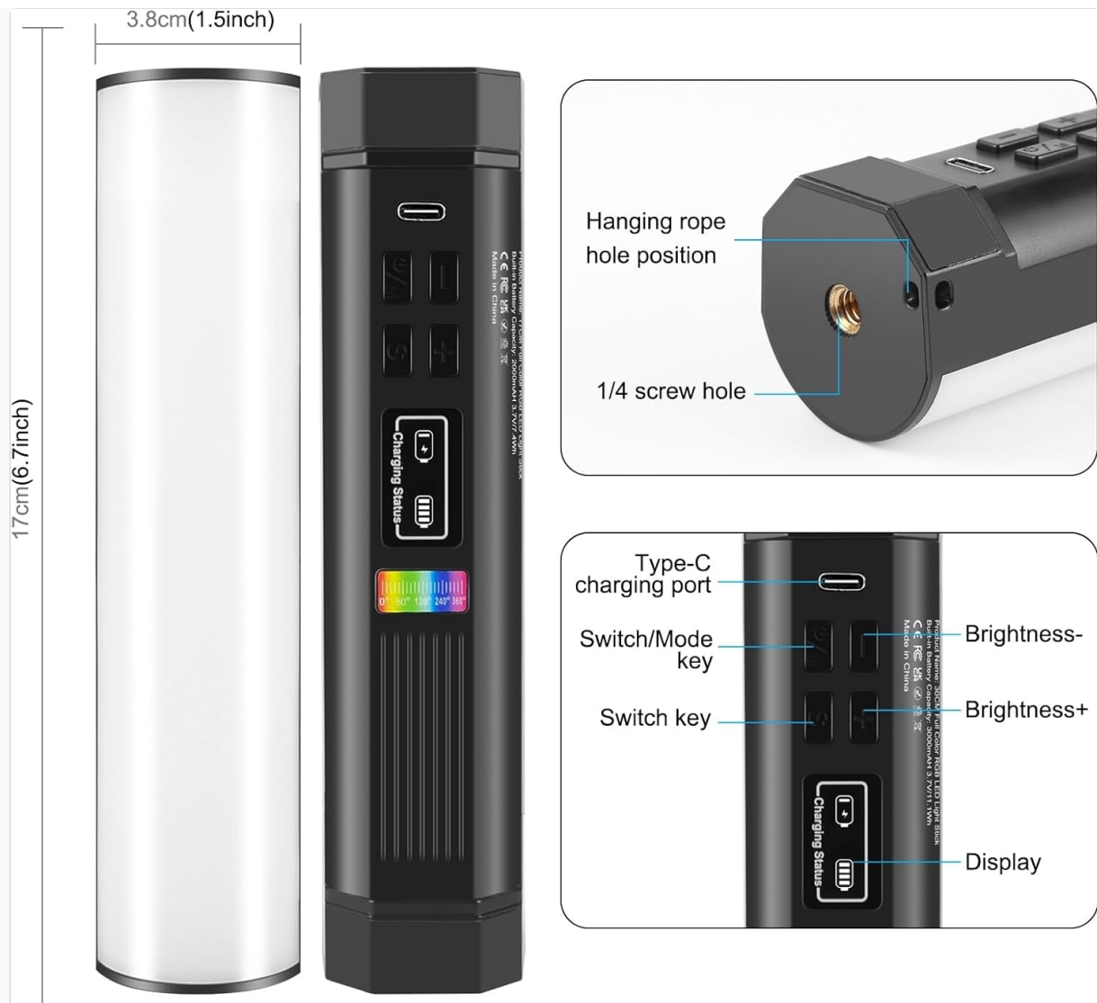
Image 4.1: Product dimensions and control layout. The light stick measures 17cm (6.7 inches) in length and 3.8cm (1.5 inches) in diameter. It features a Type-C charging port, a Switch/Mode key, Switch keys for brightness adjustment, and a display screen. Both ends include a 1/4 inch screw hole and a hanging rope hole position.
