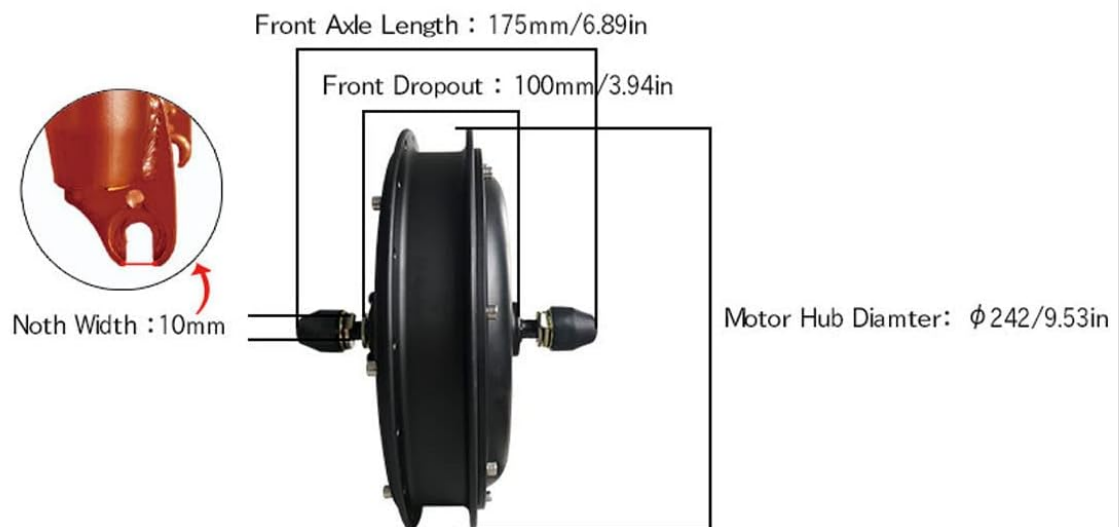
Figure 3.1: Diagram illustrating the front motor dimensions and the required 100mm front fork opening size for installation.
