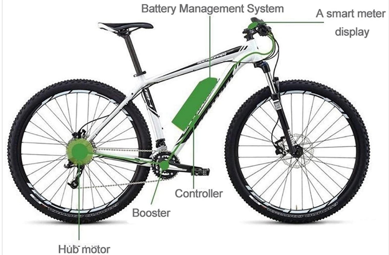
Figure 3.3: Schematic diagram showing the typical installation locations for the hub motor, controller, battery management system, smart meter display, and booster (PAS sensor) on a bicycle.
