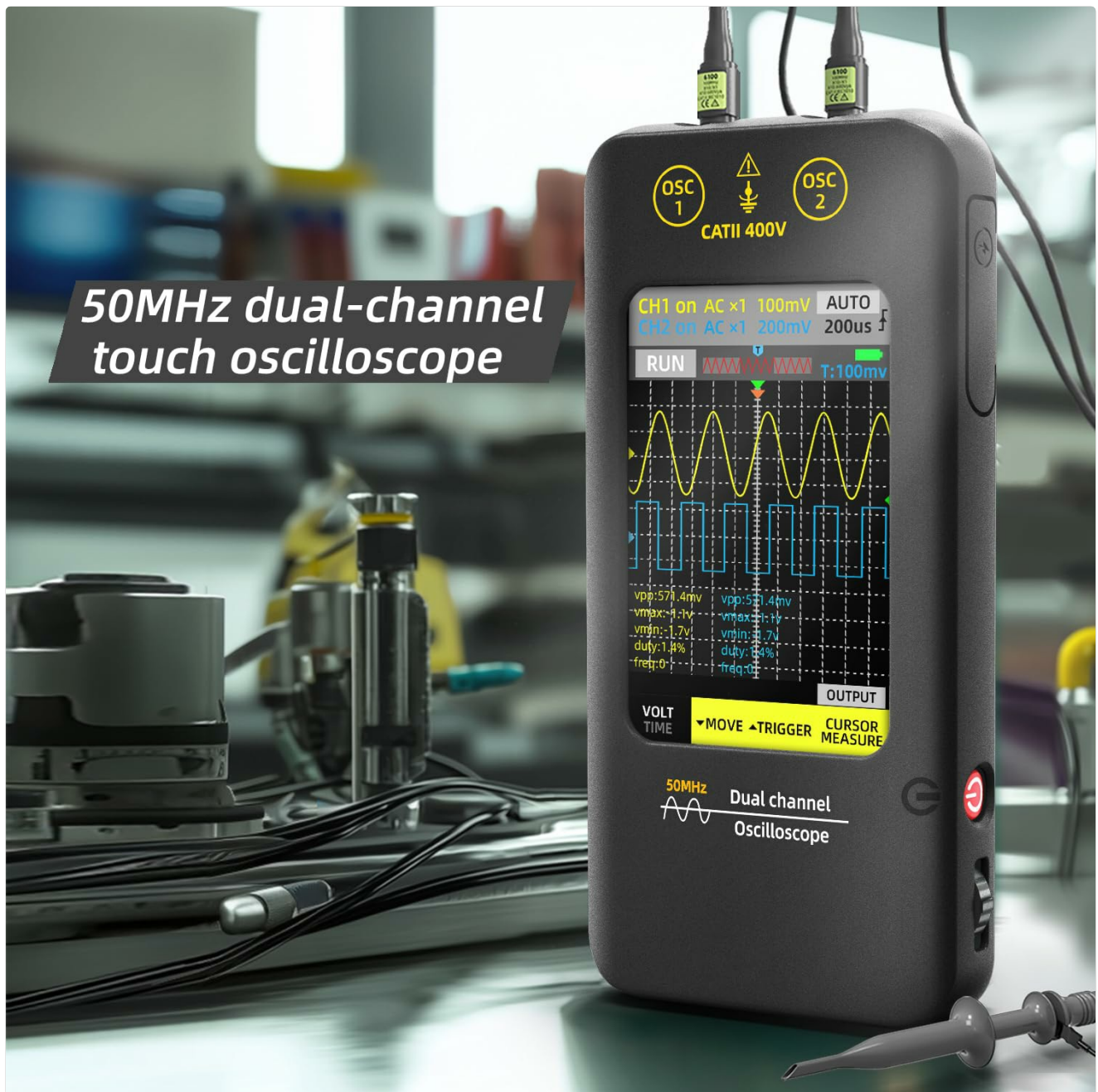
Figure 3.1: The O2 Digital Oscilloscope in an operational setting, showcasing its 50MHz dual-channel touch display and compact form factor.
