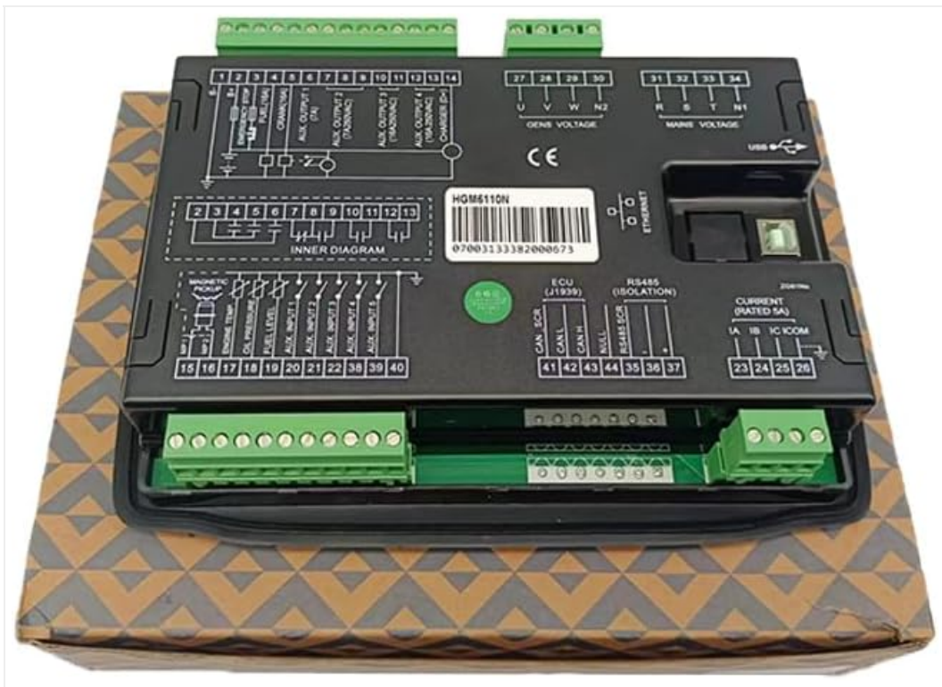
Figure 3.2: Rear view of the SmartGen HGM6110N Generator Controller, displaying the various wiring terminals for connections such as generator voltage, mains voltage, current inputs, and auxiliary outputs.
