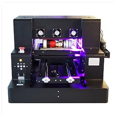
Figure 6: Printer with bottle holder for cylindrical items.
