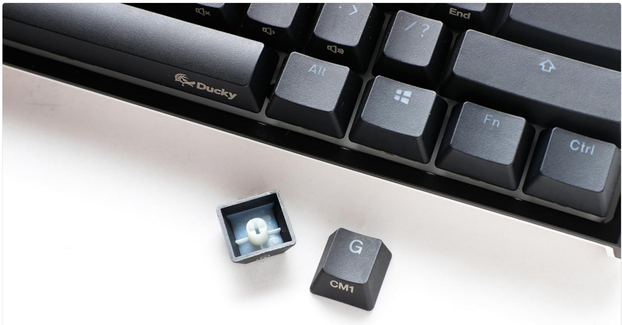
Image 5.1: A keycap removed from the Ducky One 2 Mini Pro, revealing the Gateron Red mechanical switch underneath.
