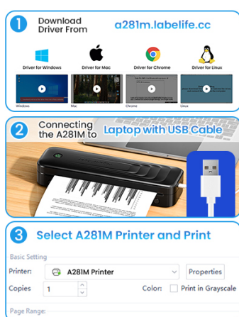
Figure 3.3: Connect your printer to a laptop or PC via USB after downloading the appropriate drivers from the provided website.
