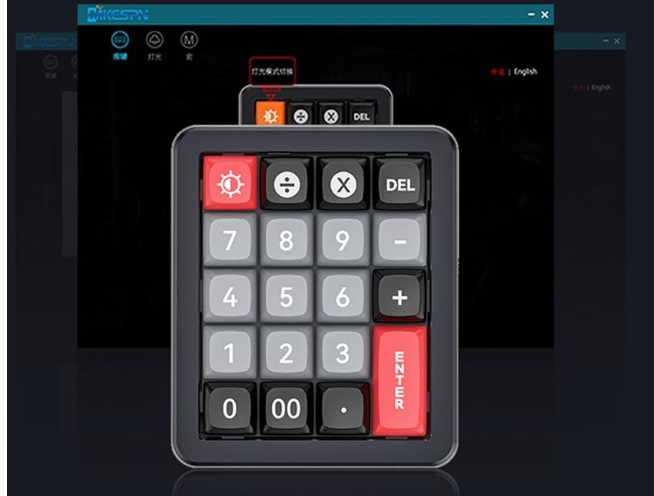
A visual representation of the macro programming software, which allows users to define custom functions and macros for the keyboard's 19 programmable keys.
