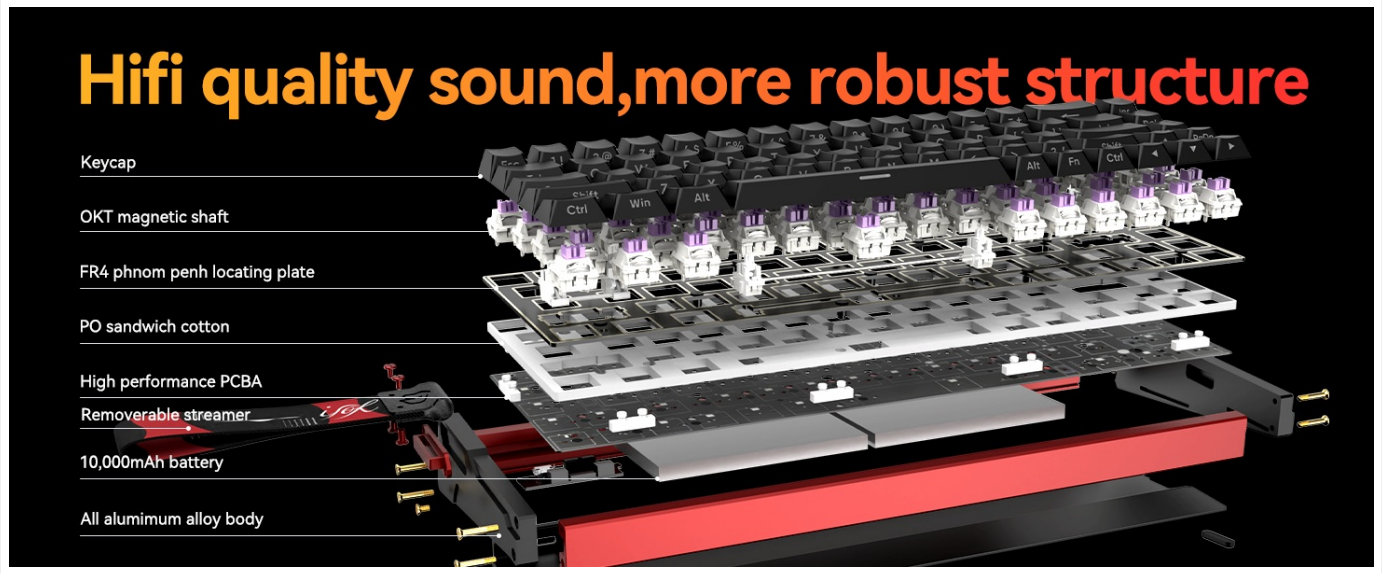
Figure 9: Internal structure of the IROK MG68, illustrating components for maintenance and customization.
