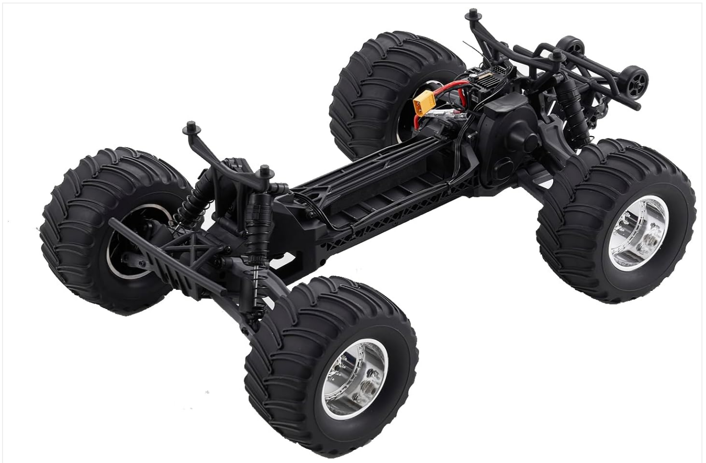
Image: The FMS 1/10 Ford F-100 chassis with electronics visible, demonstrating the internal layout before the body is attached.
