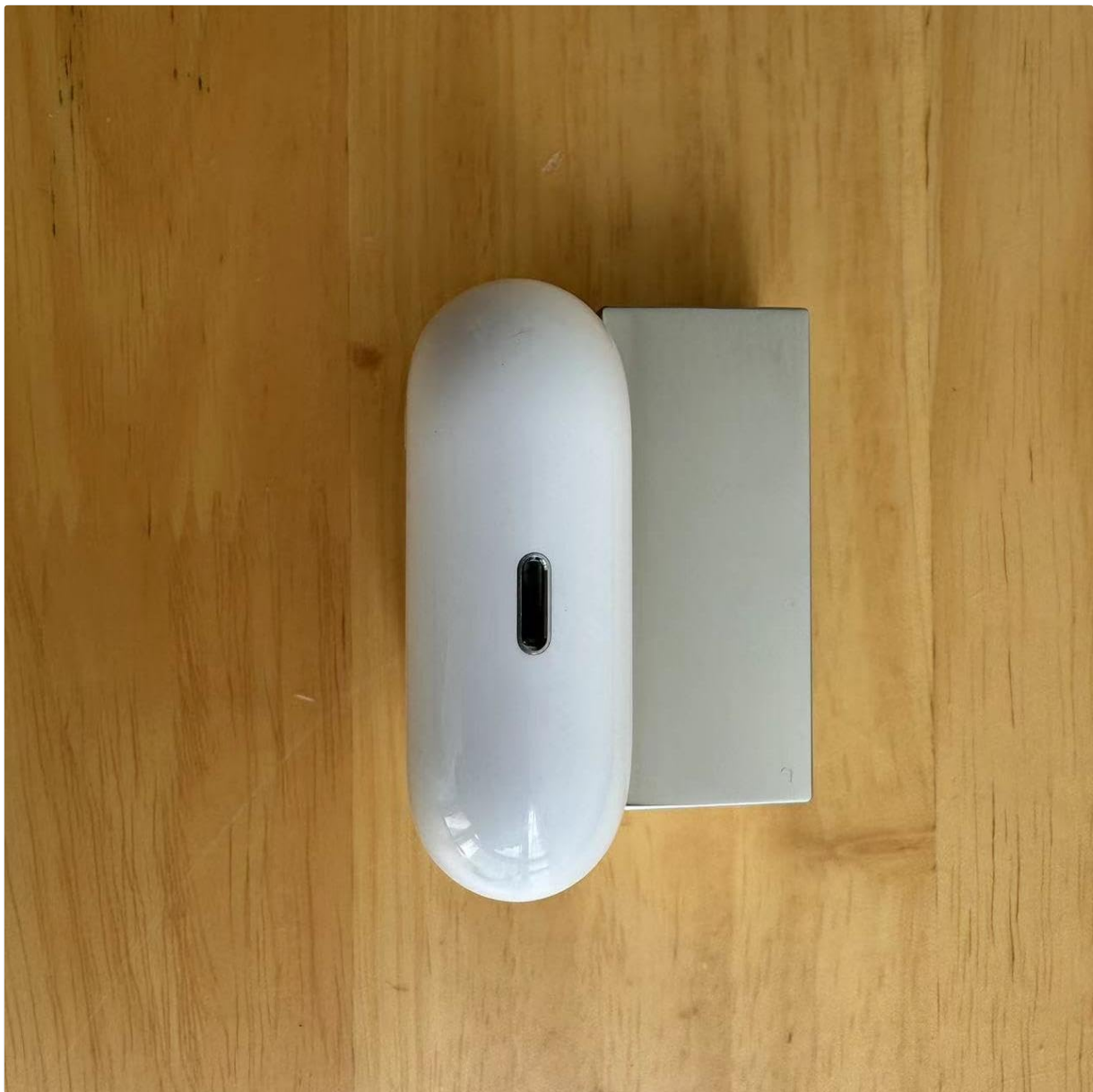
Image 4.1: The bottom of the Meenova A2190 Charging Case, illustrating the Lightning charging port.
