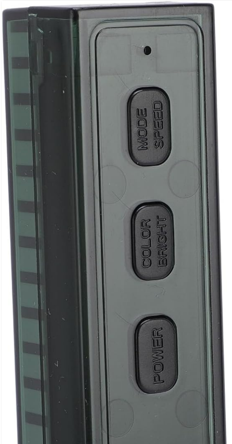
Figure 2.3.1: Side view of the light bar, highlighting the control buttons and the USB-C power input.
