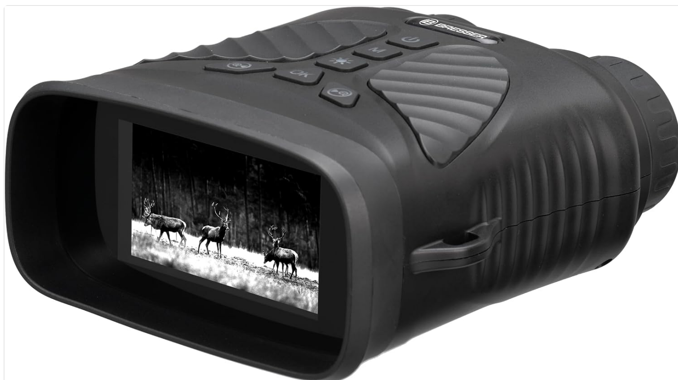
Figure 1.1: Front view of the Bresser NightSpy DT showing the display and control buttons.
