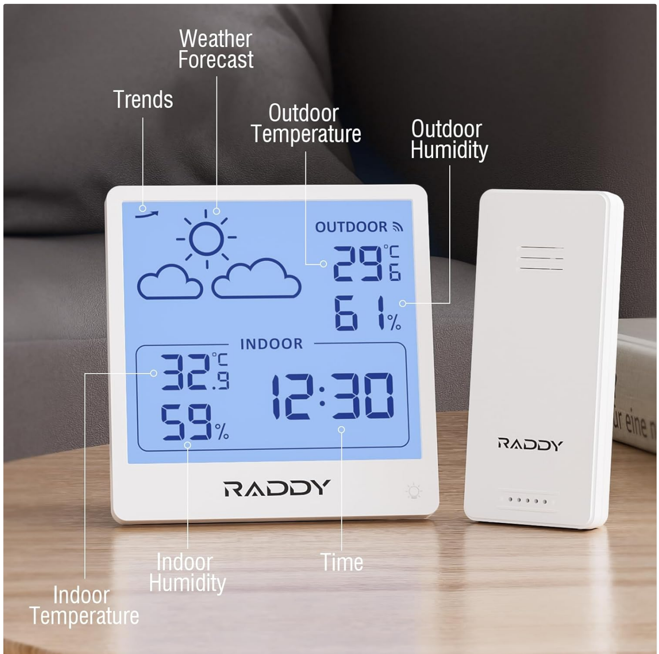
Figure 2: Detailed view of the Raddy WF-50 display showing various data points.
