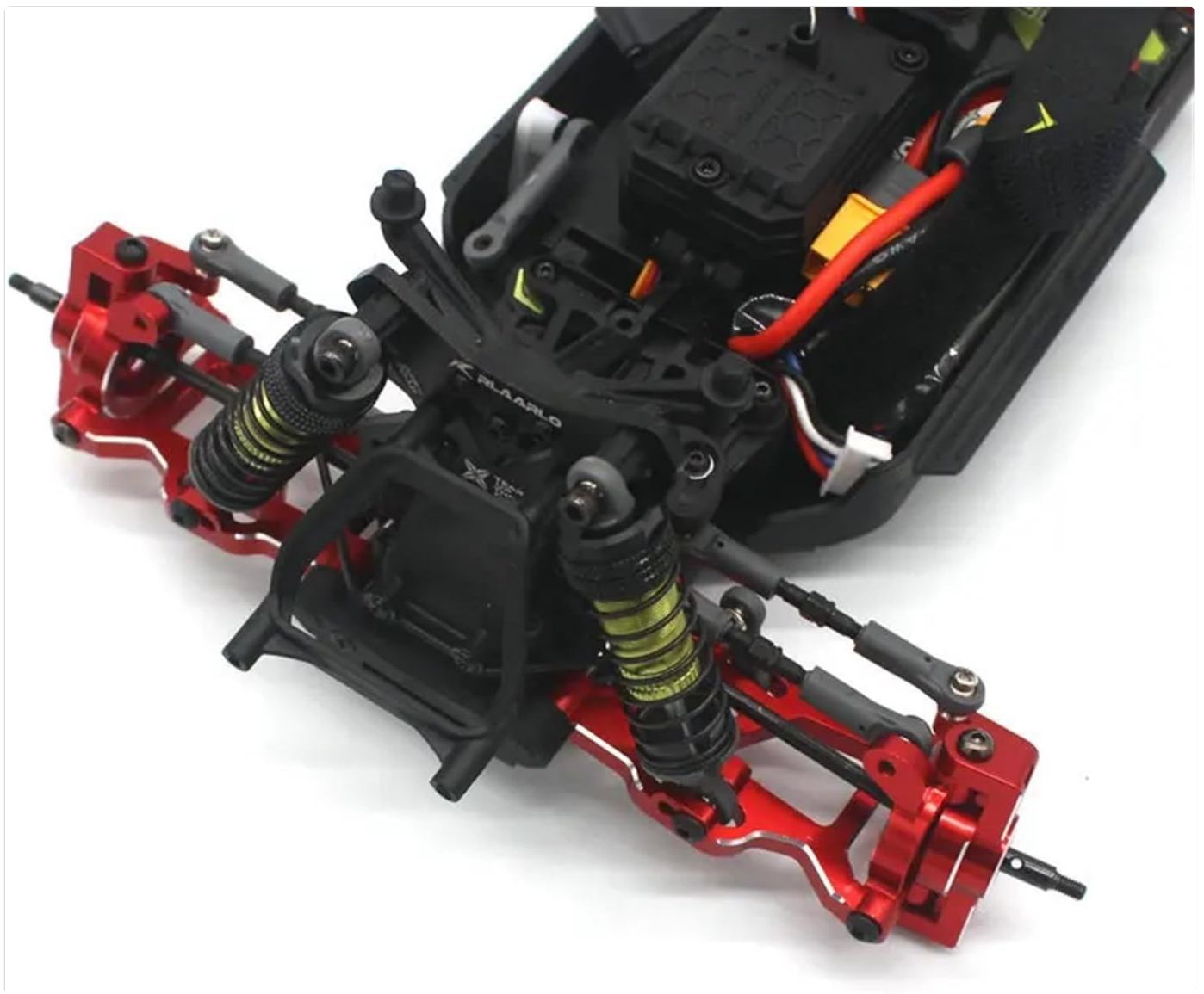
Image 3: A detailed view of an RC car's front section, showcasing the red metal swing arms and steering cups installed, highlighting their integration with the suspension and steering mechanisms.
