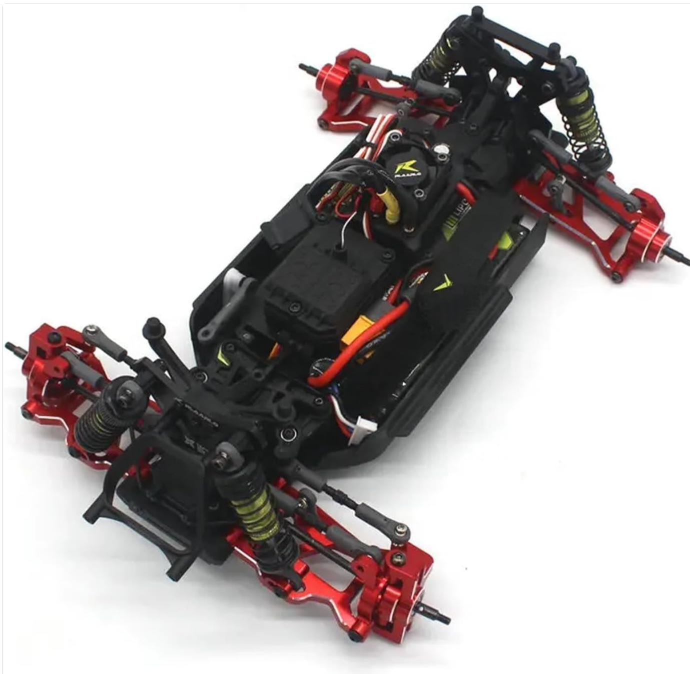
Image 4: An overhead perspective of an RC car chassis, illustrating the full installation of the red metal upgrade parts on both the front and rear suspension systems.
