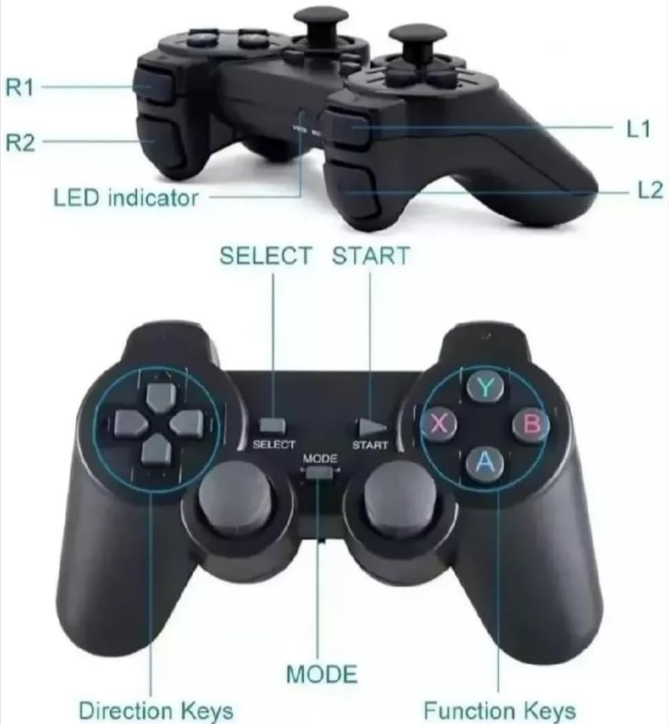
Image 5.1: Wireless Controller Layout.
