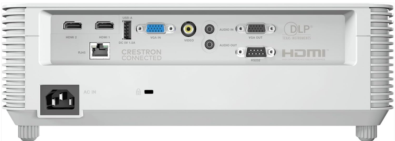
Figure 3.3: The rear panel provides various input and output ports, including HDMI, VGA, USB-A, RJ45, RS232, and audio connections.
