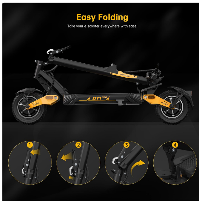
Image: A visual guide illustrating the simple steps required to fold the AUSOM Leopard DT1 Pro Electric Scooter, making it compact for storage or transportation.
