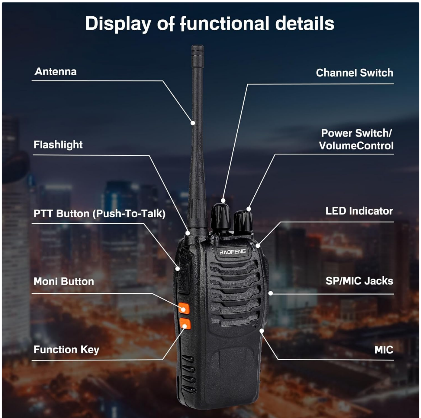
Figure 2: Functional Details of the Baofeng 888S Radio
