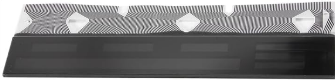
Figure 2.2: Rear view of the LCD screen display, illustrating the flexible circuit board (FPC) connections.
