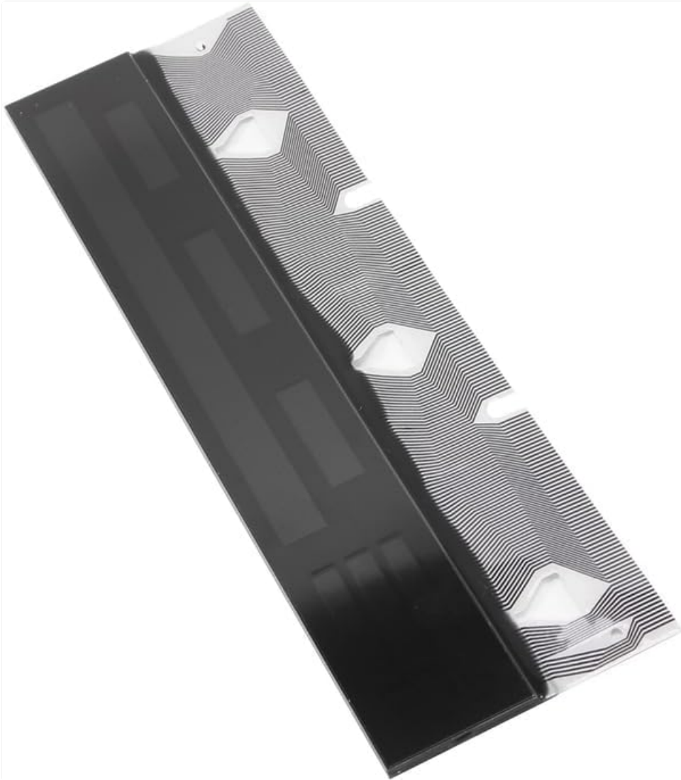
Figure 4.1: Angled view highlighting the flexible circuit board (FPC) which connects the display to the instrument cluster's main board.
