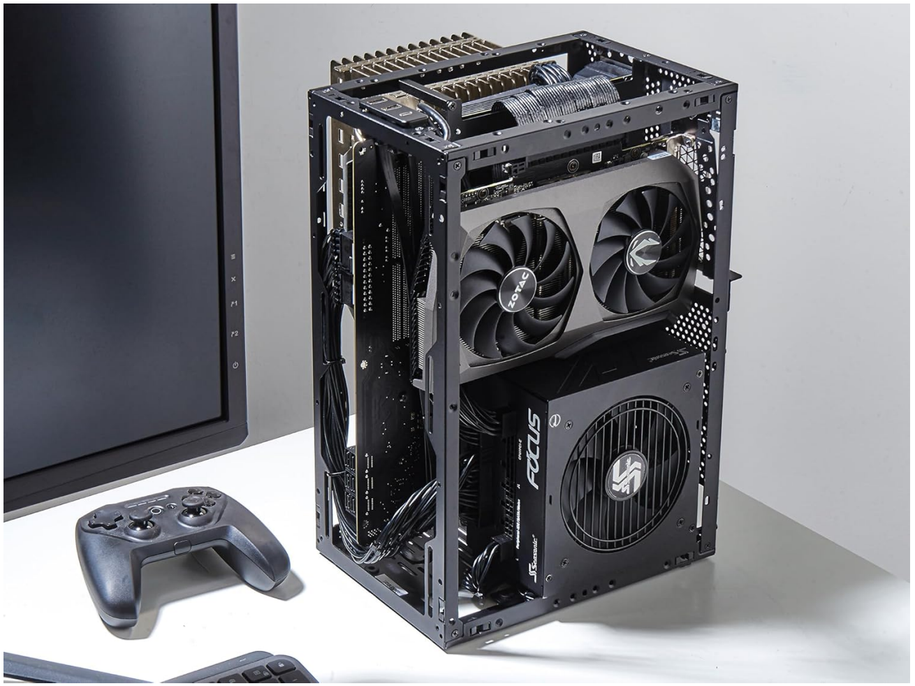
Figure 6.1: Internal view showing the power supply and GPU, areas that benefit from regular dust removal.
