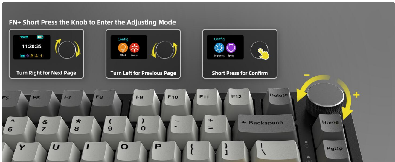
Image 3.1: The multi-function knob and TFT smart display.
