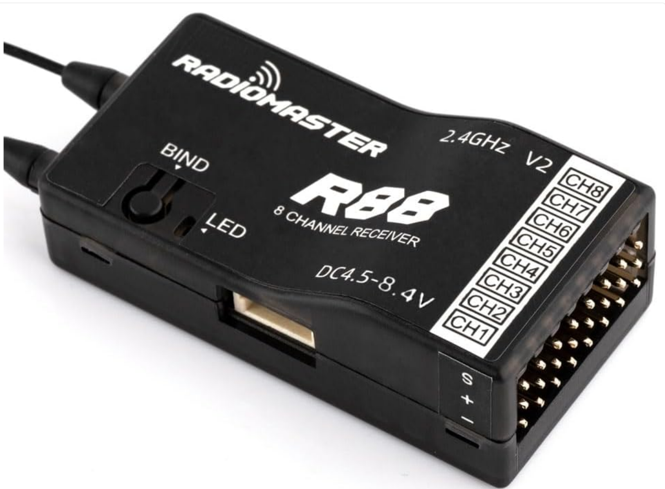
Figure 3.1: Front view of the Radiomaster R88 V2 receiver, showing the bind button, LED indicator, and channel outputs.
