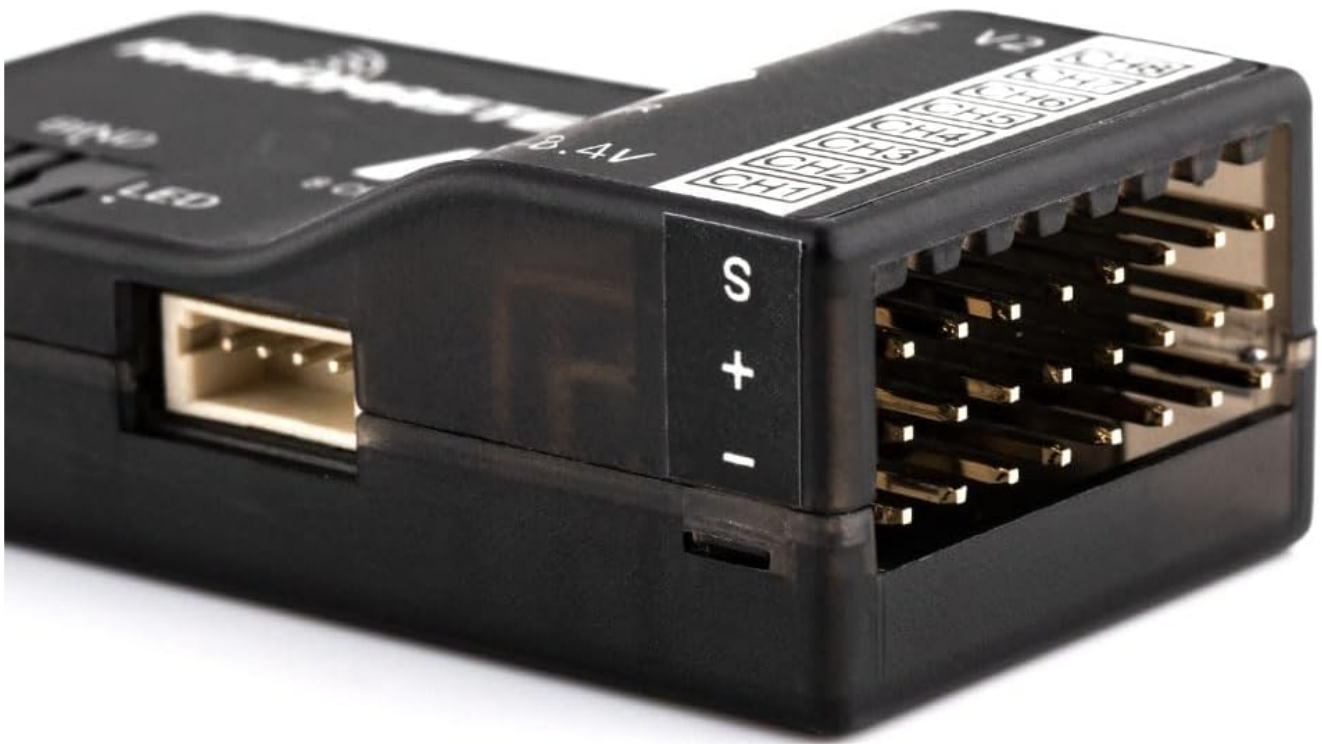
Figure 3.4: Close-up view of the R88 V2 receiver's channel and Sbus ports.
