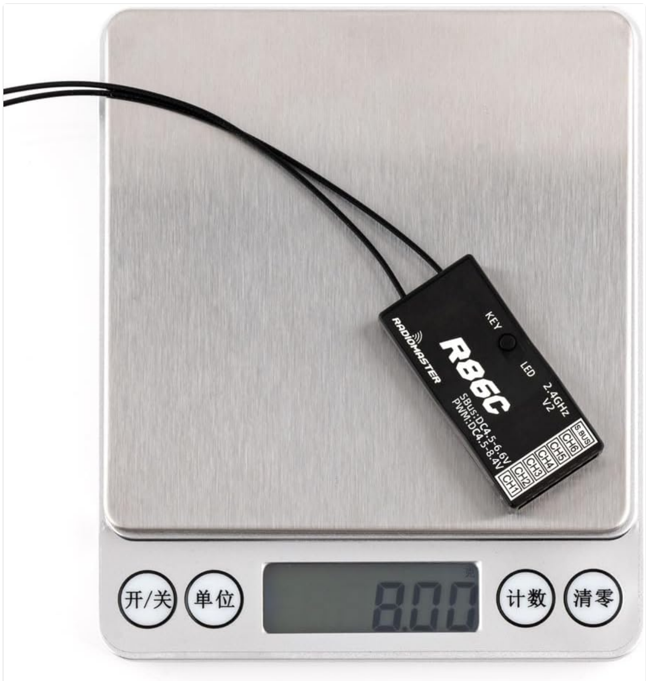
Image 4.2: The Radiomaster R86C V2 receiver placed on a digital scale, displaying a weight of 8.00 grams.
