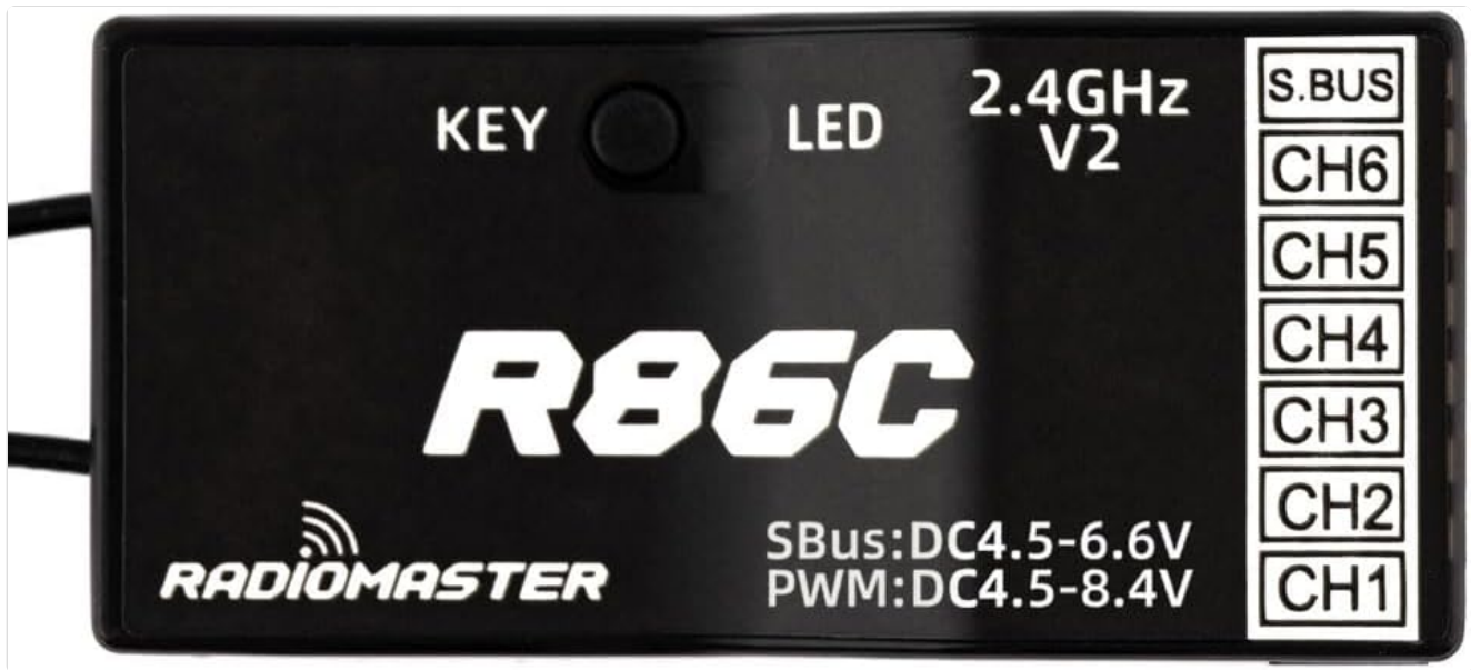
Image 3.1: Front view of the Radiomaster R86C V2 receiver, showing the KEY button, LED indicator, 2.4GHz V2 label, and channel outputs (S.BUS, CH6-CH1).
