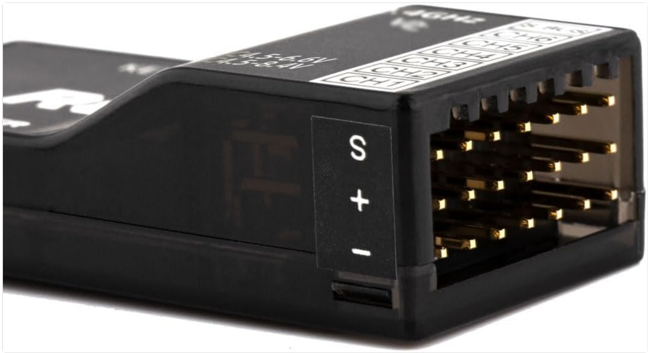
Image 5.1: Close-up view of the receiver's pin headers, showing the 'S', '+', and '-' labels for signal, positive power, and negative power connections, respectively.
