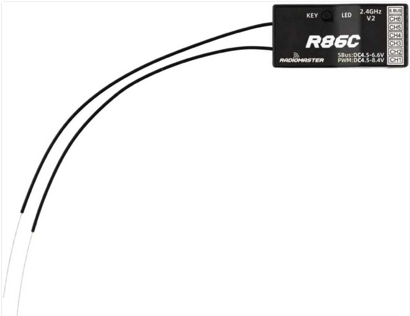
Image 3.2: The Radiomaster R86C V2 receiver with its dual antennas extended, illustrating the full setup for optimal signal reception.
