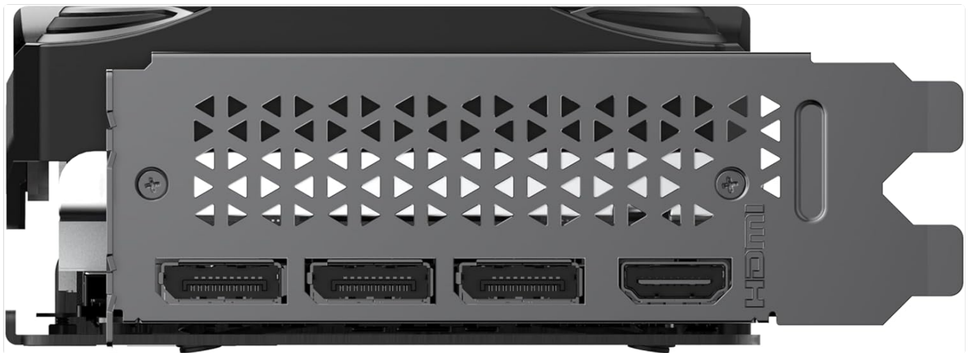
Figure 3.2: Display output ports on the graphics card.
