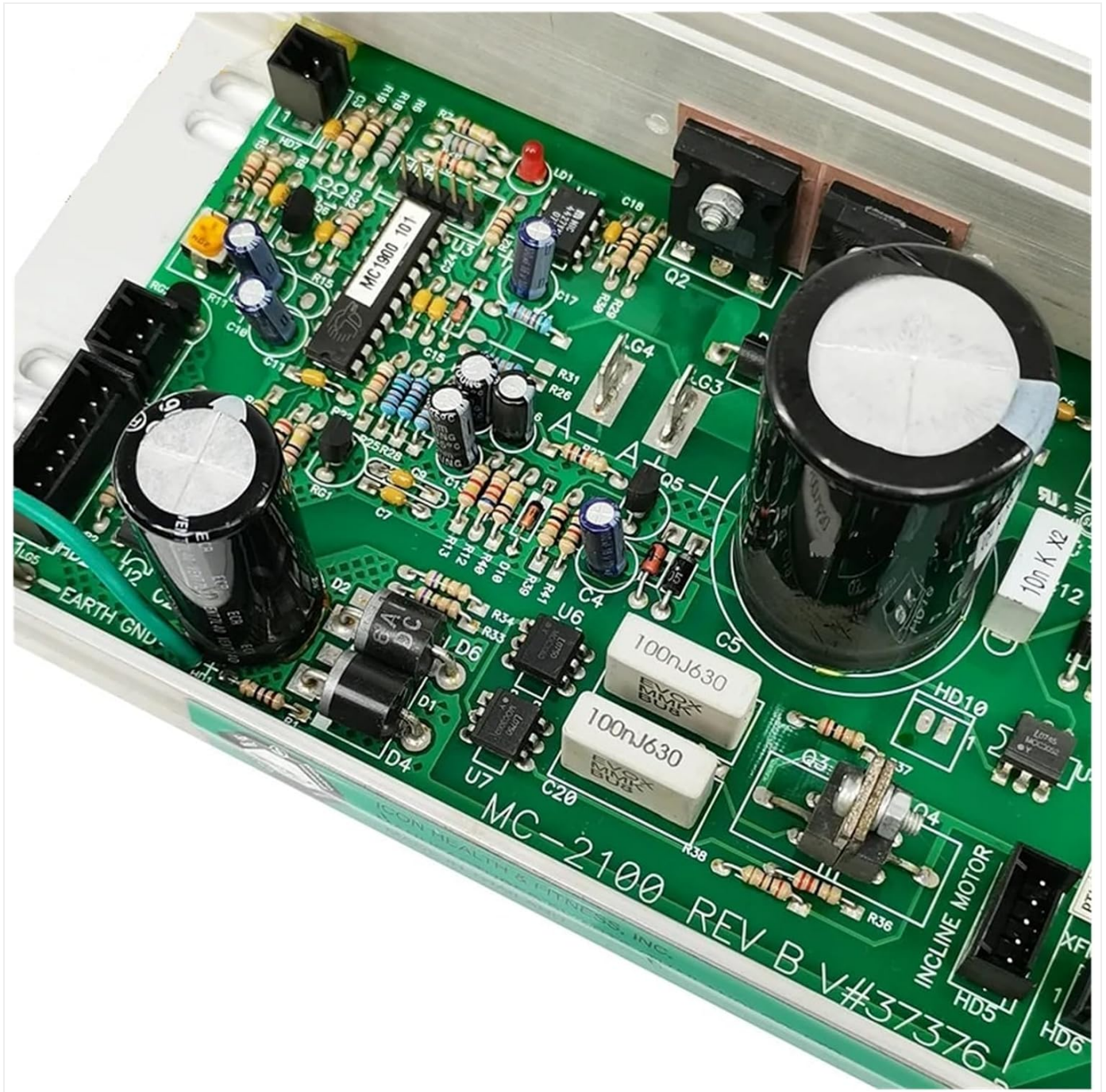
Figure 3: Detailed view of the MC-2100 REV B circuit board, highlighting various integrated circuits, capacitors, and resistors. Proper connection points for motor, AC input, and other signals are visible.
