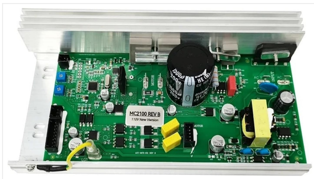
Figure 1.1: Top view of the MC-2100 REV B Treadmill Controller, showing various electronic components and heat sink.
