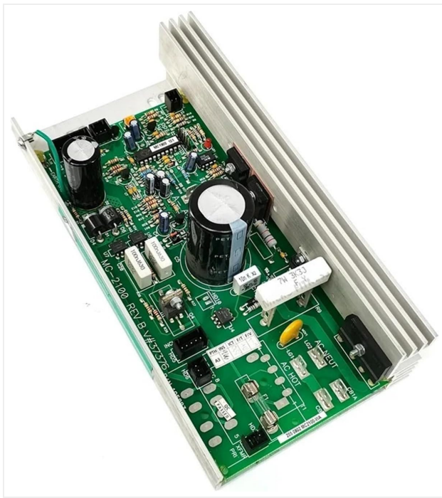
Figure 1.2: Angled perspective of the MC-2100 REV B controller, highlighting the side heat sink and component layout.
