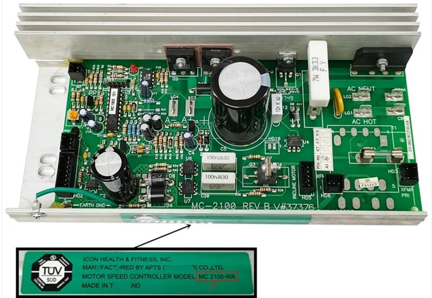
Figure 4: The MC-2100 REV B / MC2100-WA controller, confirming its model and 110V compatibility, along with a TUV SUD certification mark.
