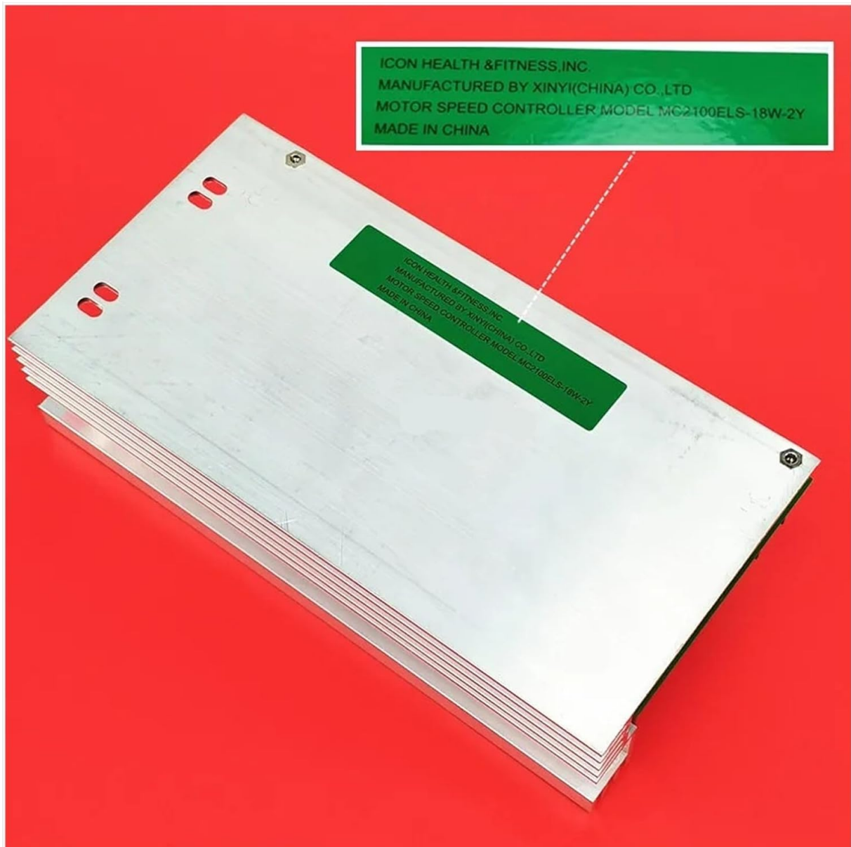
Figure 2.1: Top view of the SBJKBVMF MC2100ELS-18W-2Y Treadmill Motor Controller. This image shows the aluminum heat sink and the green label indicating the model number and manufacturer.
