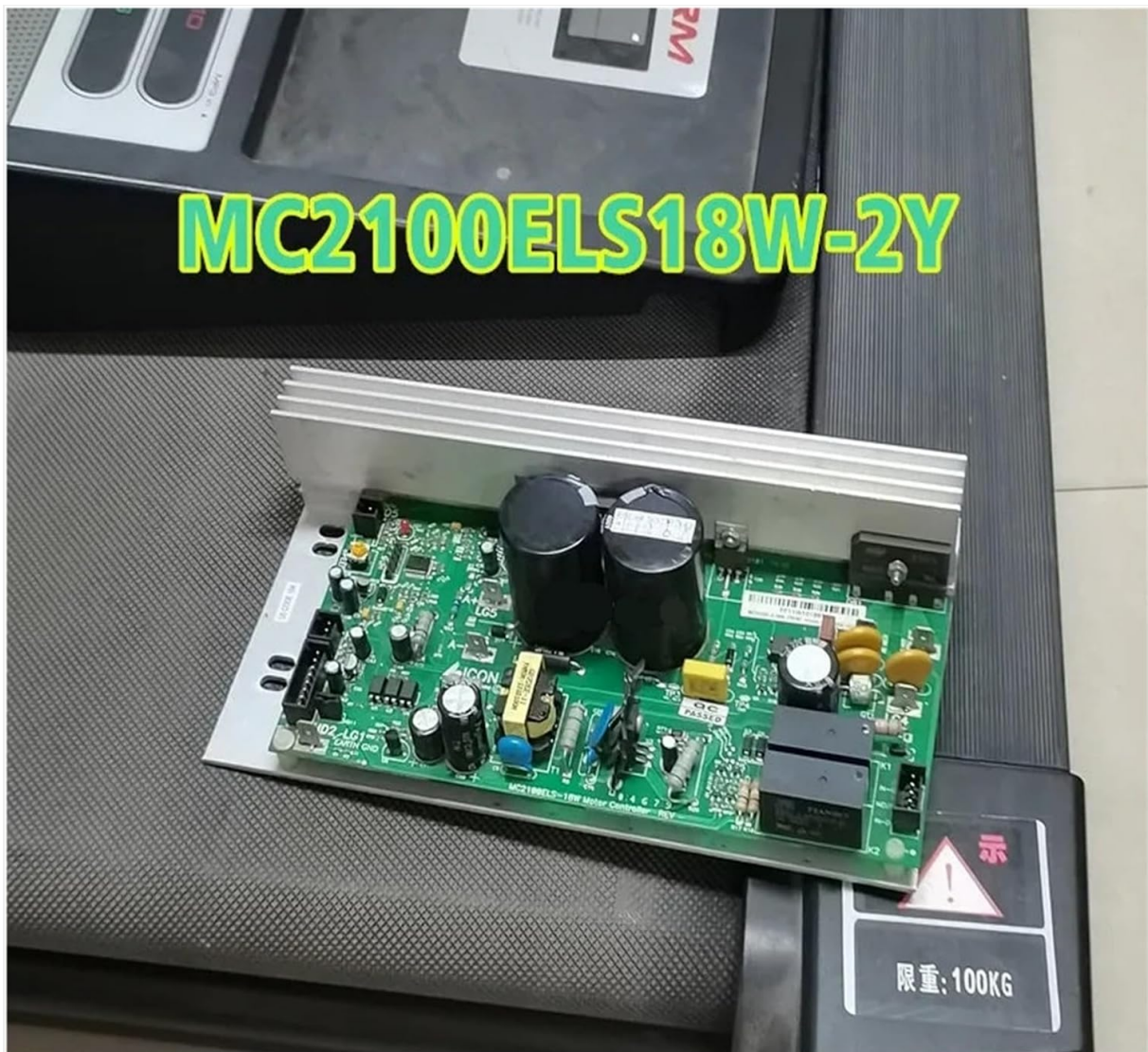
Figure 3.2: The SBJKBVMF MC2100ELS-18W-2Y controller installed within a treadmill's motor compartment. This image provides a visual reference for the placement of the controller in a typical treadmill setup.
