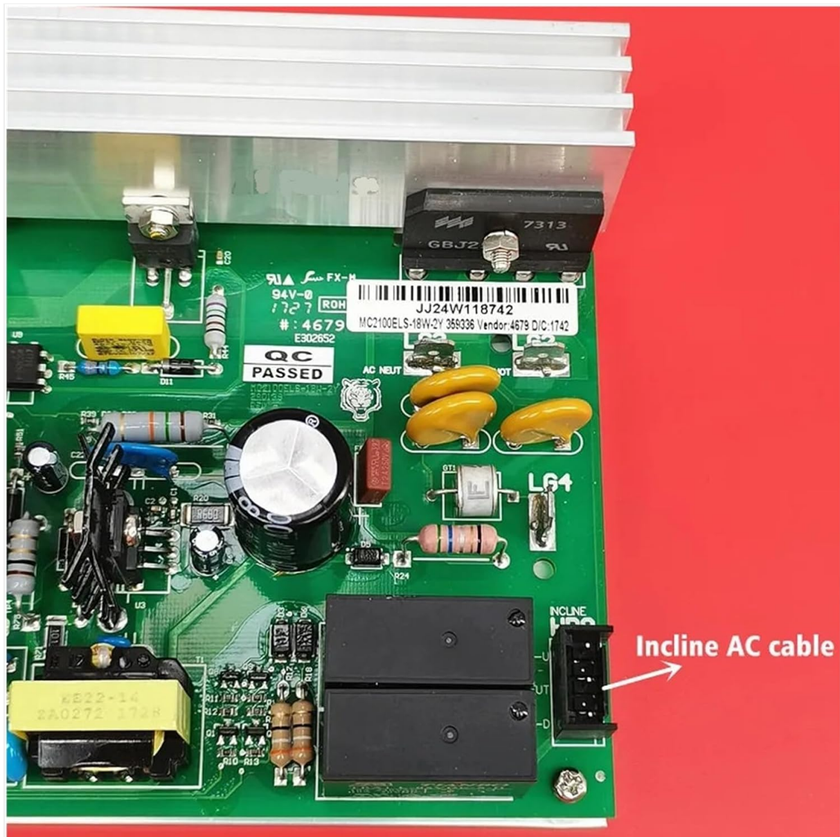
Figure 3.1: Close-up view of the incline AC cable connection point on the treadmill motor controller. This image highlights the 'Incline AC cable' connector, which is a critical connection during installation.
