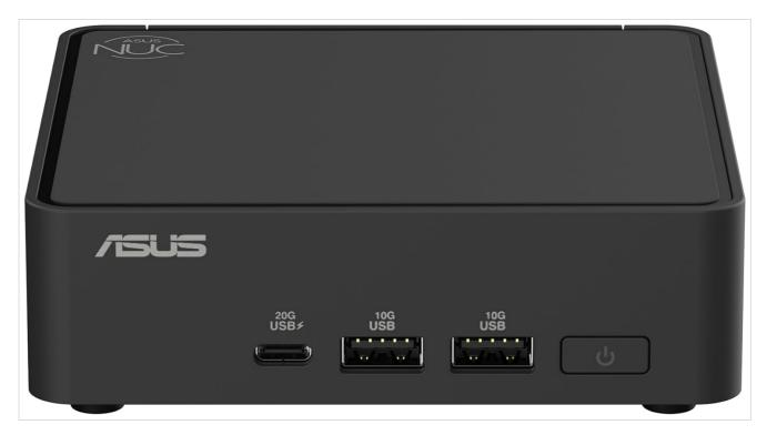
**Image:** Front view of the ASUS NUC 15 Pro Slim PC Kit, showing the ASUS NUC logo on top, ASUS branding on the front, and various USB ports and the power button. From left to right, a USB-C 20G port, two USB-A 10G ports, and the power button.
