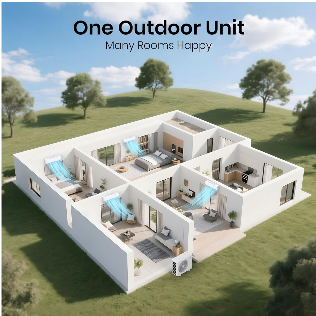
Image 3.1: Illustrates the multi-zone capability, where a single outdoor unit efficiently serves multiple indoor units, providing independent climate control for different rooms.
